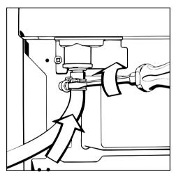
Detach the hose clip from the drain outlet at the back of the machine and remove the rubber plug.  Push the drain hose onto the drain outlet. Make sure that the hose is firmly secured by the clip and not kinked.
